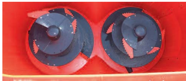
The polygonal shape of the hopper acts as a brake, holding the material for longer to increase the rate of chopping. Details such as the pitch of the auger coils and positions of knives on the auger all contribute to more efficient processing of long fibre.
